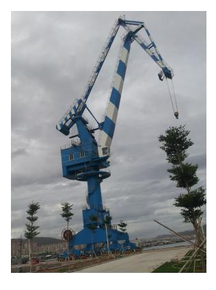
**Double boom portal jib crane** is used to build ship as indispensable lifting equipment, they requires a light or medium working grade (A7 or A8) for double boom crane.
